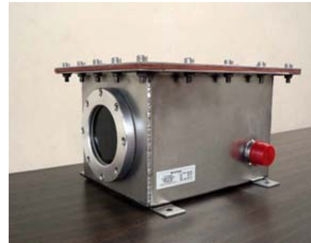
Wave Height Sensor In Explosion Proof Stainless Steel Enclosure
